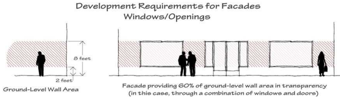
Figure: Development requirements for facades windows/openings
