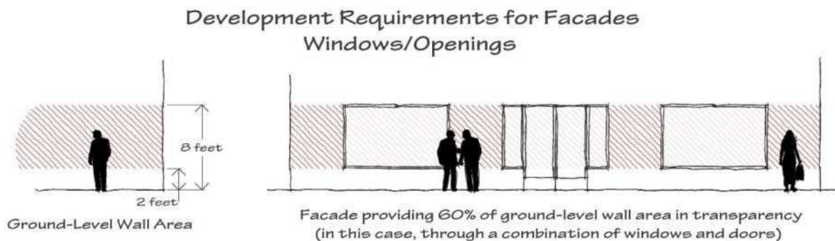
Figure: Development requirements for facades windows/openings
