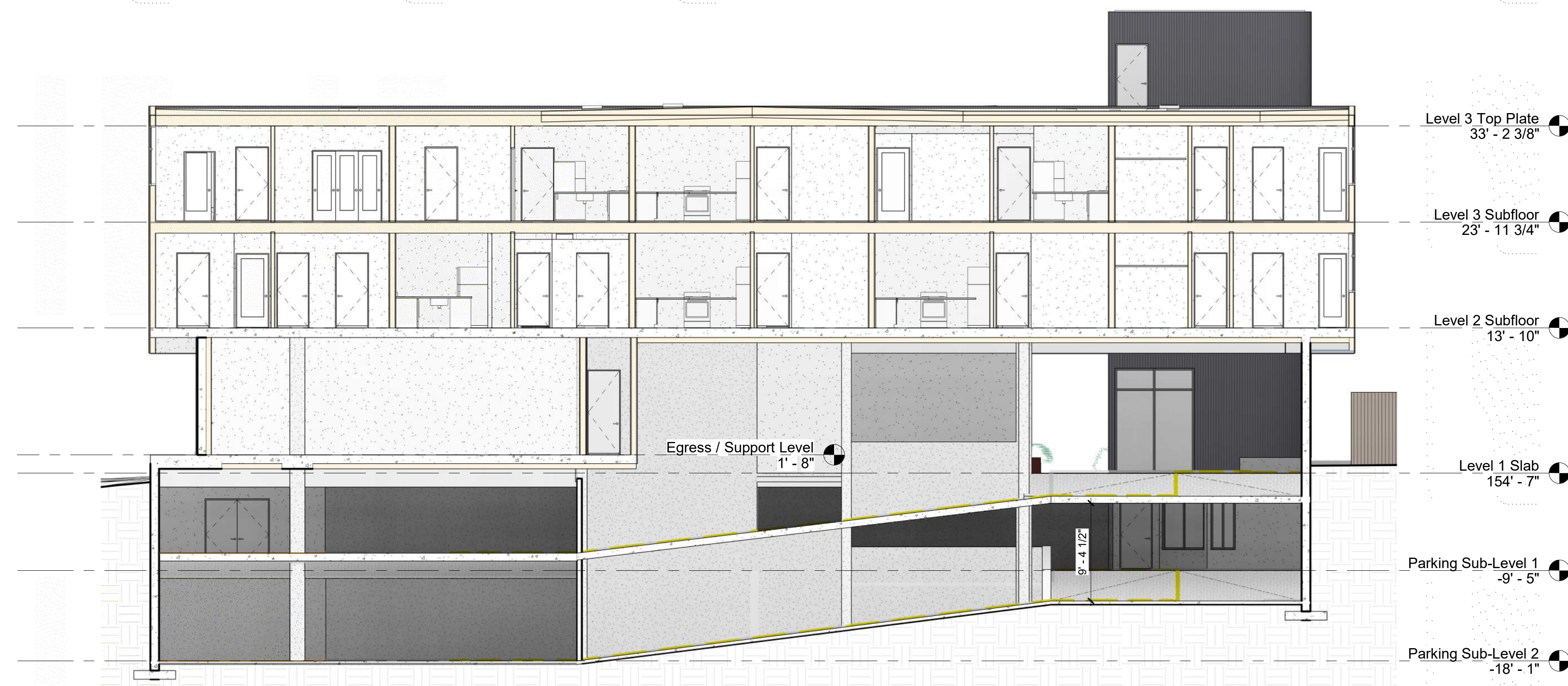
① N-S Through Garage Ramps 1/8" = 1'-0"
